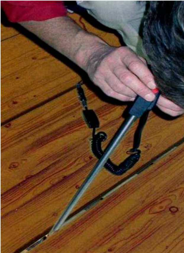
An endoscope being used to investigate beneath floorboards.
